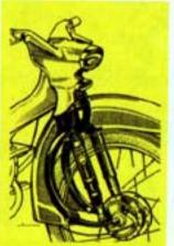
Fabulously Comfortable Riding Due to the spring travel of 82 m/m front and 90 m/m at the rear. Quickly-I riders only see potholes on the rood - they never feel them. Taut long swinging arms at the front and a swinging fork rear suspension are a first-class combination and they represent the experience which NSU designers have occumulated throughout many years. Four hydroulic shock obsorbers hidden away in four telescopic legs give the Quickly-T considerable road holding properties.
