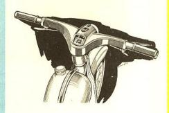
Even in the dreariest places riders on the Quickly-L have a pleasing sight before their eyes: the pressed steel section handlebar, which is absolutely up-to-date in shape and equipment. The best thing is the three-in-one combination: headlamp, handlebar and speedometer (with milometer) built into one unit. Another thing: the tangle made up of cables and electric wires has completely disappeared into the channel, so that it is protected from the wet and from meddling fingers.
